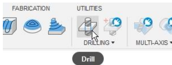
Figure 42. Create a Drill operation
