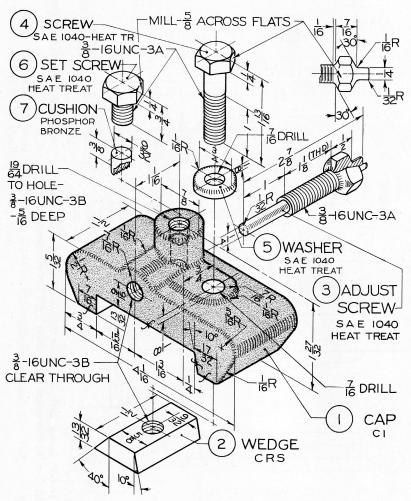
Fig. 14-65 Clamp Stop. (1) Draw details. (2) Draw assembly.
