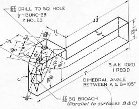
Fig. 8-49 RH Tool Holder. Draw necessary views, including partial auxiliary views showing 105° angle and square hole true size. For threads, see §§13.15 and 13.16 (Layout B-4).
