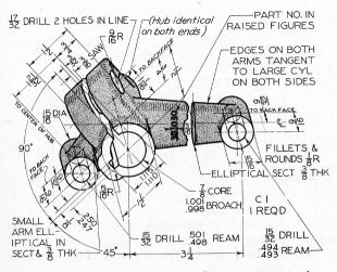
Fig. 8-46 Brake Control Lever. Draw necessary views and partial views (Layout B-4).
