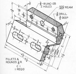
Fig. 8-48 Cam Bracket. Draw necessary views or partial views as needed. For threads, see §§13.15 and 13.16 (Layout B-4).
