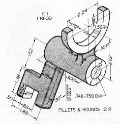
Fig. 8-47 Shifter Fork. Draw necessary views, including partial auxiliary view showing true shape of inclined arm (Layout B-4).
