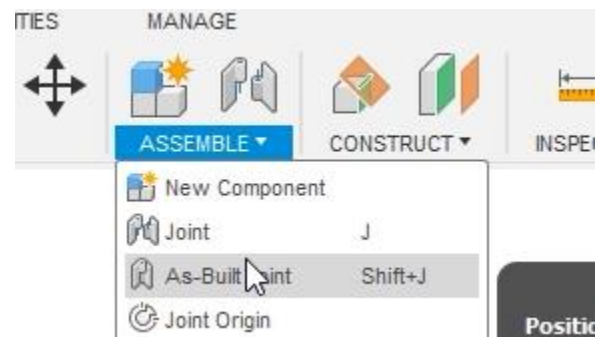
Figure 12. Open the As-Built Joint tool
