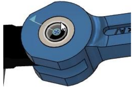
Figure 20. Create a new As-Built Joint
