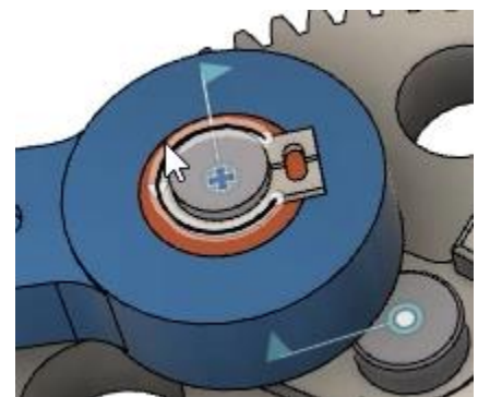
Figure 19. Create a new As-Built Joint
