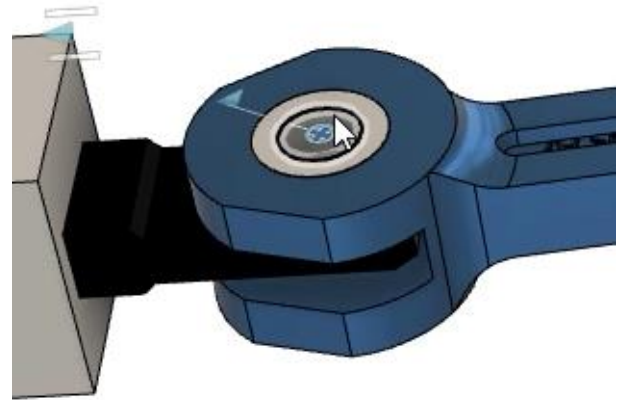
Figure 26. Re-create the necessary joints
