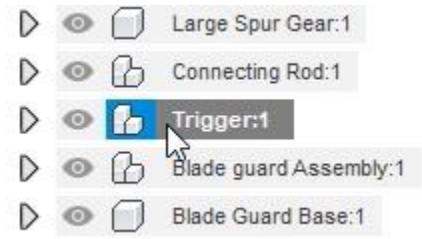
Figure 4. Unground the Trigger component
