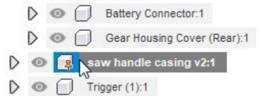
Figure 3. Ground the saw handle casing
