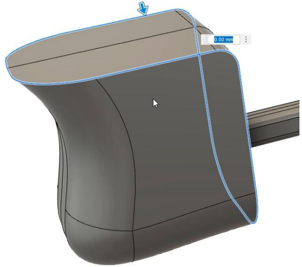
Figure 16. Fillet two more edges
