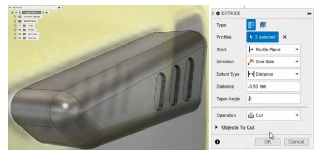
Figure 13. Extrude cut slot geometry
